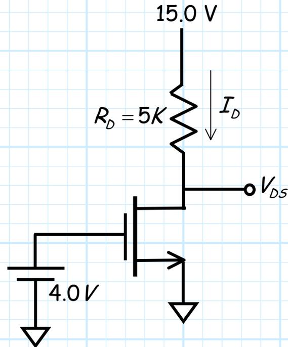
Thus, the DC voltage  $V_{DS}$  can be determined from *KVL* as:
