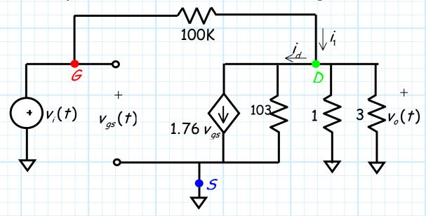
We find first that  $v_{gs} = v_i$ . We likewise see from KCL that current  $i_1$  is:
