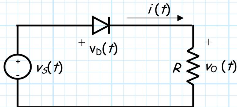
Let's use the **CVD model** to determine the output voltage  $v_O$  in terms of the input voltage  $v_s$ . In other words, let's determine the diode circuit **transfer function**  $v_O = f(v_s)$ !
