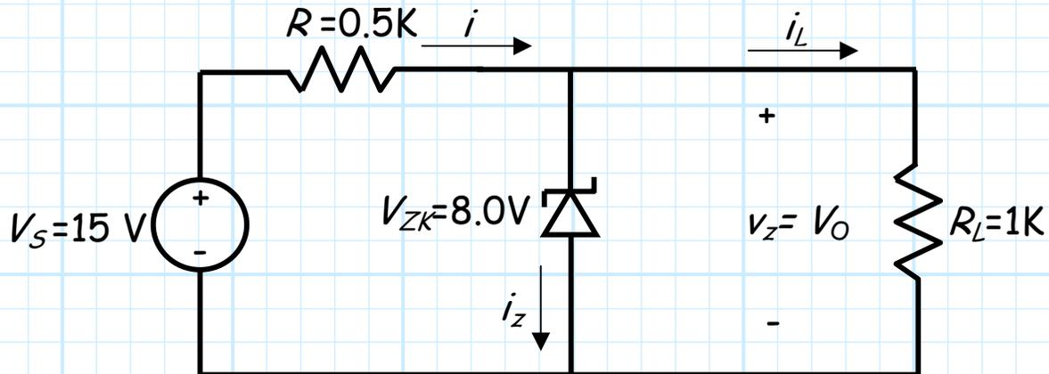
Note that the load resistor  $R_L$  is in **parallel** with the Zener diode, so that the voltage  $V_O$  across this load resistor is **equal** to the Zener diode voltage  $v_Z$ .
