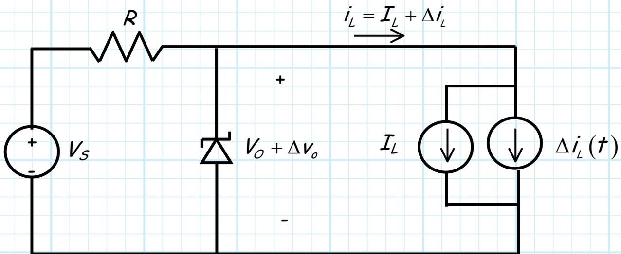
**Q:** Just how are  $\Delta i_L$  and  $\Delta v_o$  related? I mean, if  $\Delta i_L$  equals, say,  $50 \text{ mA}$ , what will value of  $\Delta v_o$  be?
