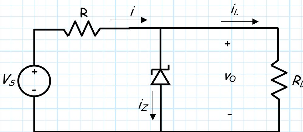
For voltage regulators, we typically define a load  $R_L$  in terms of its current  $i_L$ , where:
