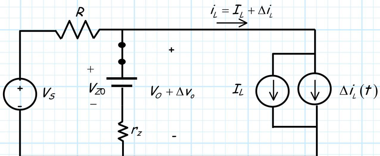
We then turn **off** all the **DC** sources (including  $V_{Z0}$ ) and analyze the remaining **small-signal circuit!**
