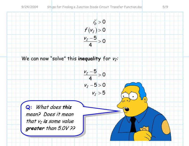
A: NO! Recall that  $v_I$  can be **any** value. What the inequality above means is that  $i_D^{i} > 0$  (i.e., the ideal diode is forward biased) WHEN  $v_D^{i} > 5.0$ .
