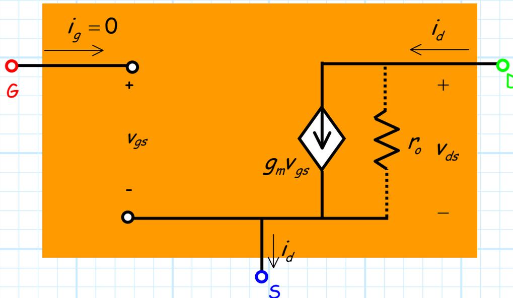
Therefore, replacing a MOSFET with its small-signal circuit model is very simple—you simply change the stuff **within** the orange box!
