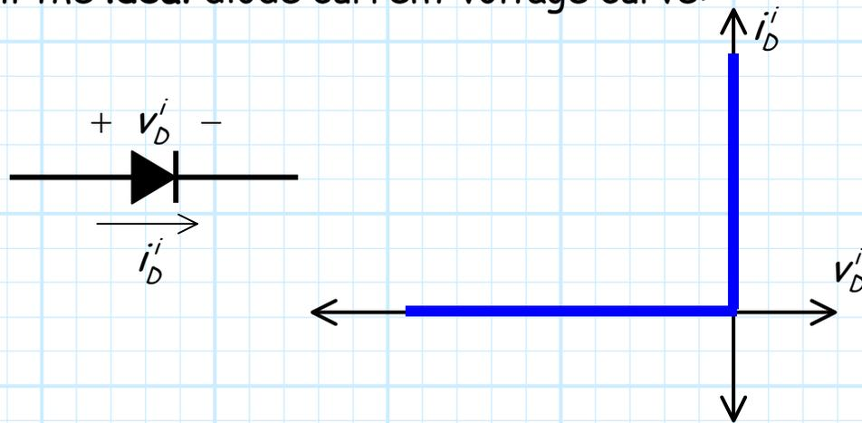
This curve is piece-wise linear, with two **unambiguous** regions—**reverse** bias (where  $v < 0$  and  $i = 0$ ), and **forward** bias (where  $i > 0$  and  $v = 0$ ).
