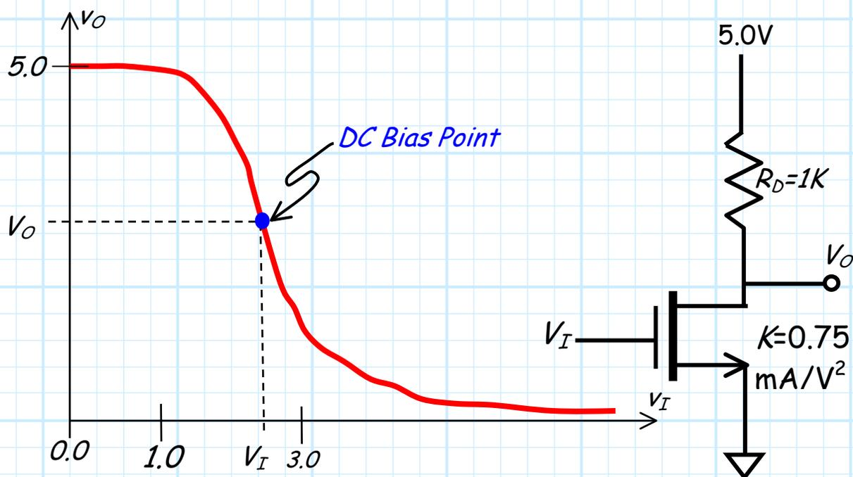
Now, say we **add** a **small-signal**  $v_i$  to this input DC voltage (i.e.,  $v_I(t) = V_I + v_i(t)$ ). This small signal simply represents a small change in the input voltage from its **average** (i.e., DC) value. The result is of course as **small change** in the **output** voltage—the **small-signal output voltage**  $v_o(t)$ !
