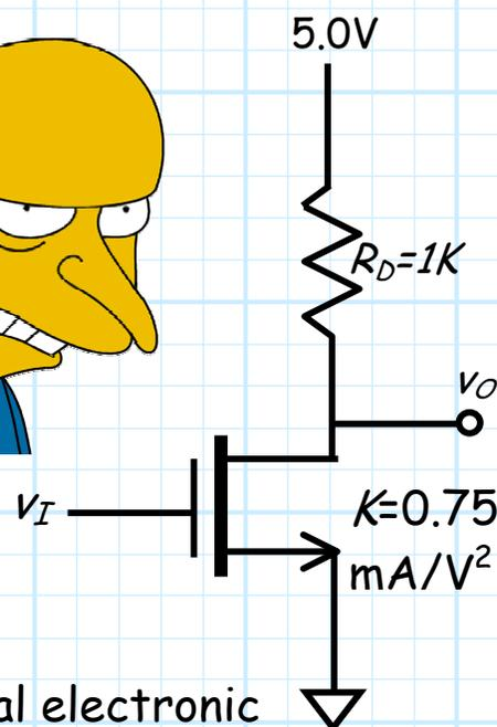
**A:** Actually, this circuit is a fundamental electronic device! To see what this circuit does, we need to determine its **transfer function**  $v_O = f(v_I)$ .
