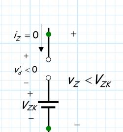
Analyzing this Zener CVD model, we find that **if** the model voltage  $v_Z$  is less than  $V_{ZK}$  (i.e.,  $v_Z < V_{ZK}$ ), then the **ideal** diode will be in **reverse** bias, and thus the model current  $i_Z$  will equal **zero**. In other words:
