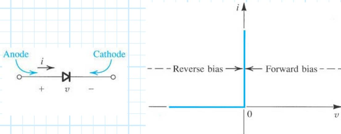
This curve is piece-wise linear, with two **unambiguous** regions—**reverse** bias (where  $v < 0$  and  $i = 0$ ), and **forward** bias (where  $i > 0$  and  $v = 0$ ).
