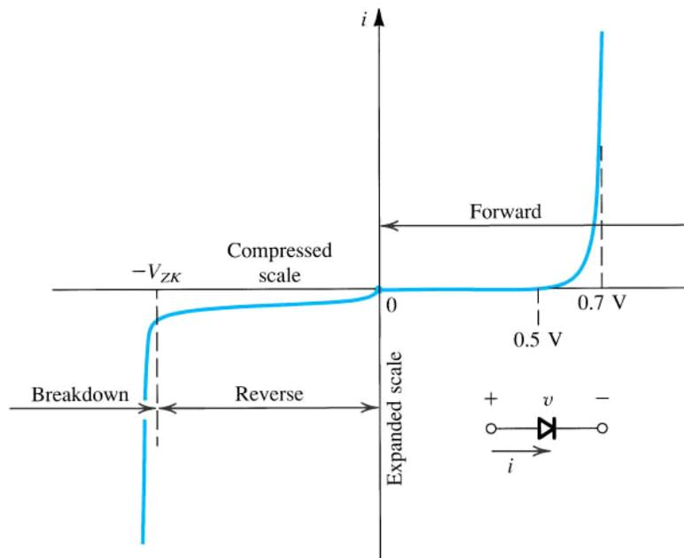
Note that the breakdown region occurs when the junction diode voltage (from anode to cathode) is **approximately** less than or equal to a voltage value  $-V_{ZK}$ . The value  $V_{ZK}$  is known as the **zener breakdown voltage**, and is a fundamental performance parameter of any **junction** diode.
