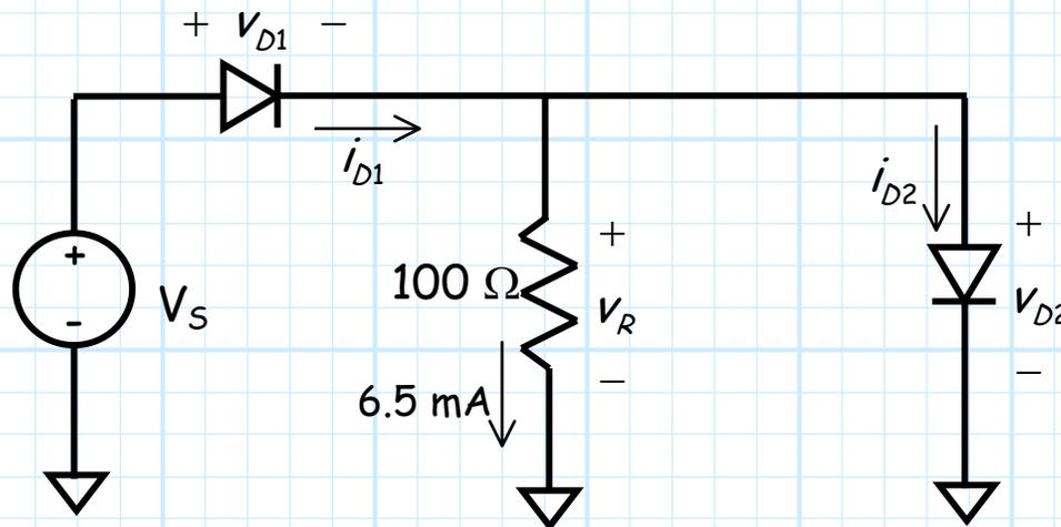
The diodes are identical, with  $n = 1$  and  $I_S = 10^{-14}\ \text{A}$ .
