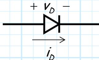
HO: The Junction Diode Curve
