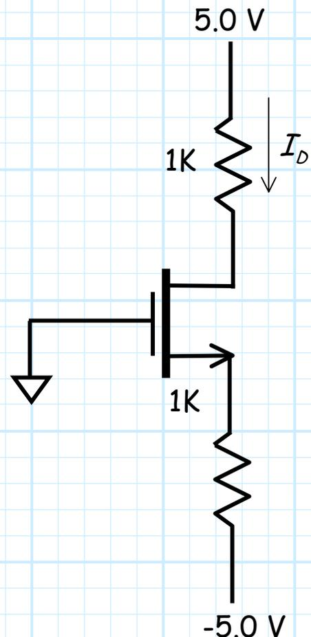
Look! We can equate the NMOS device equation and G-S equation to find  $V_{GS}$ .
