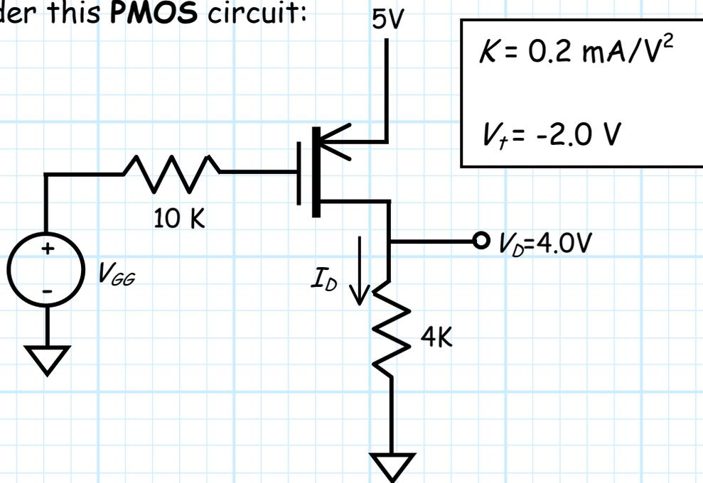
For this problem, we know that the **drain voltage**  $V_D = 4.0\text{ V}$  (with respect to ground), but we do **not** know the value of the voltage source  $V_{GG}$ .
