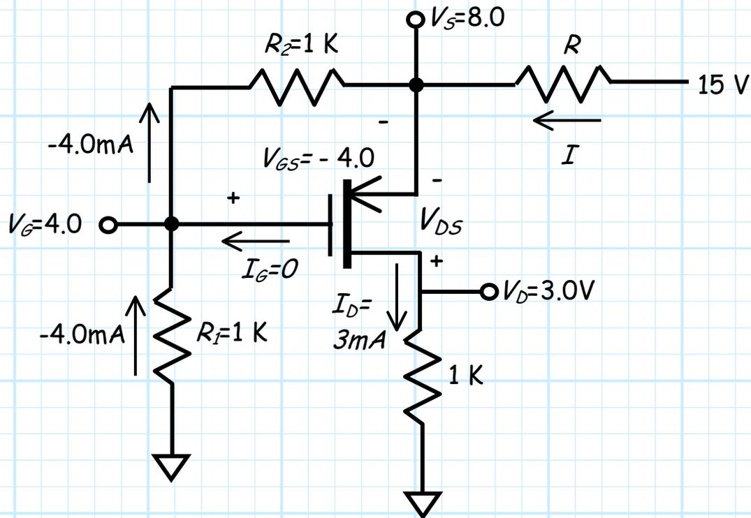
Likewise, from KCL, we can determine the current through resistor  $R$ :
