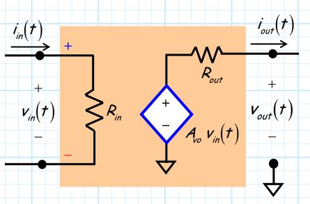
Note that **output** voltage is defined with respect to **ground** potential, while the input voltage is simply the potential **difference** between the **plus** (+) terminal and the **minus** (-) terminal.
