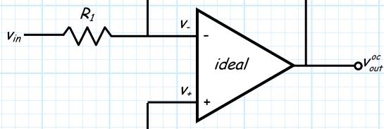
The open-circuit voltage gain of this amplifier:
