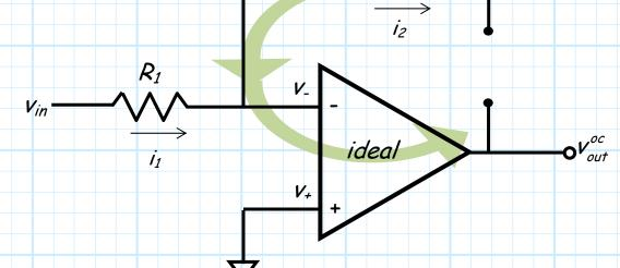
Combining, we find the open-loop gain of this amplifier to be:
