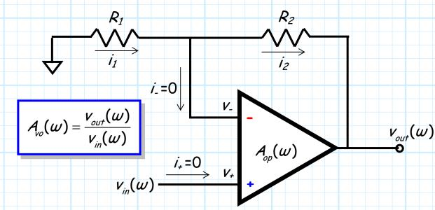
We know that the open-circuit voltage gain (i.e., the closed-loop gain) of this amplifier **should** be:
