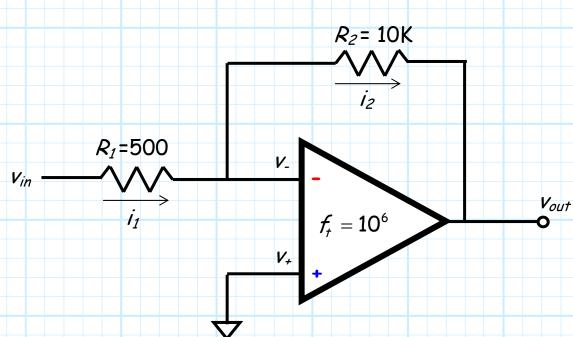
The op-amp in this circuit happens to have a unity-gain bandwidth of 1MHz.
