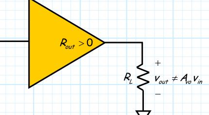
But, recall that the output voltage will be **approximately equal** to the opencircuit voltage **if** the output resistance is much **smaller** than the load resistance. I.E.,:
