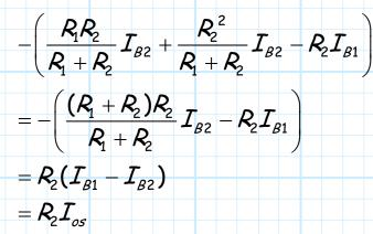
Typically, the bias currents  $I_{B1}$  and  $I_{B2}$  are approximately equal, so that **offset** current  $I_{B1} - I_{B2} = I_{os}$  is very tiny.
