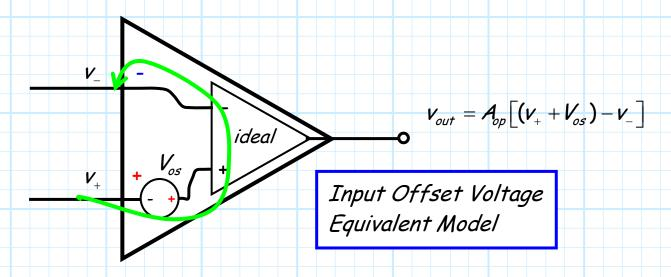
Applying the concept of a virtual short to the ideal op-amp, we find from KVL
