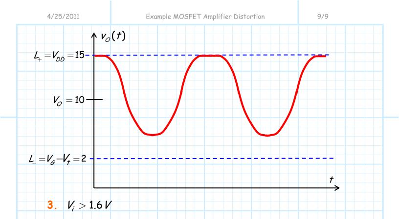
In this case, the small-signal input signal is sufficiently large so that the total output will attempt to exceed **both** limits (i.e.,  $V_{DD} = 15.0$  V and  $V_G - V_f = 2.0$  V). Therefore, there are periods of time when the MOSFE will be in **cutoff**, and periods when the MOSFET will be in **saturation**.
