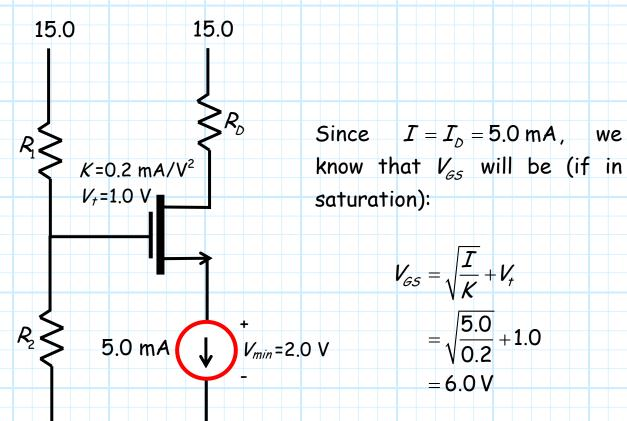
Assuming that we want the DC source voltage to be the minimum value of  $V_s = 2.0$ , we nee for the DC gate voltage to be:
