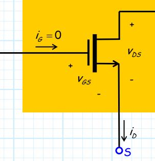
Now, **contrast** the MOSFET with its small-signal circuit model. A MOSFET small-signal circuit model is:
