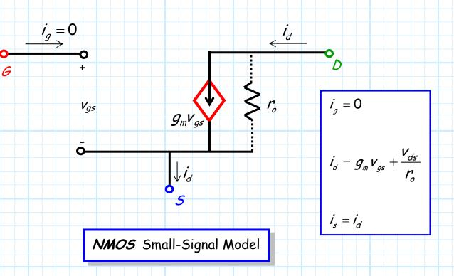
Note that this circuit provides **precisely** the same circuit equations as did our small-signal MOSFET analysis.
