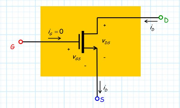
Now, contrast the MOSFET with its small-signal circuit model.
