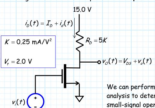
We can perform a small-signal analysis to determine the small-signal open-circuit voltage gain  $A_o$ :
