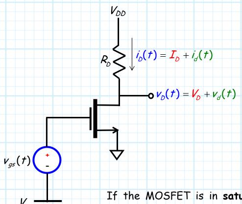
If the MOSFET is in saturation, then the total drain current is:
