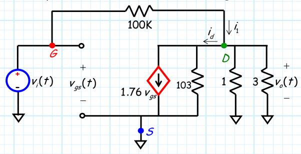
We find first that  $v_{gs} = v_i$ . We likewise see from KCL that current  $i_1$  is:
