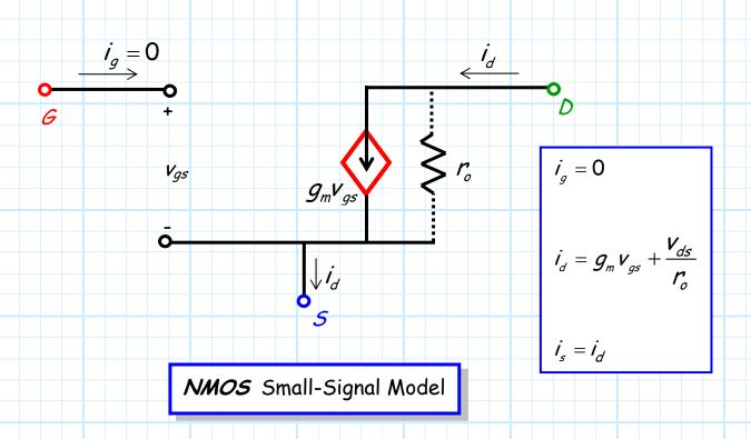
Note that this circuit provides **precisely** the same circuit equations as did our small-signal MOSFET analysis.
