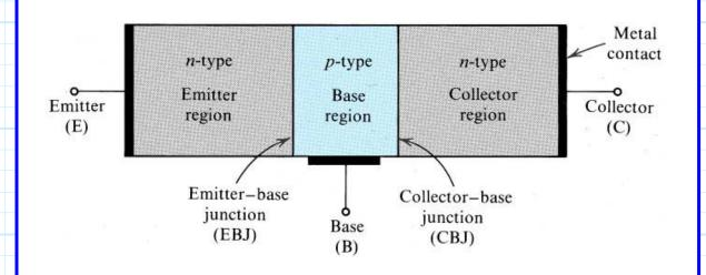
Each of the **three Silicon regions** has one terminal electrode connected to it, and thus the *npn* BJT is a **three terminal** device.
