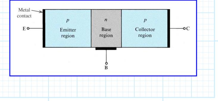
Thus, the *pnp* BJT **likewise** has **three** terminals (with the same names as the *npn*), as well as **two** *p-n* junctions (the CBJ and the EBJ).
