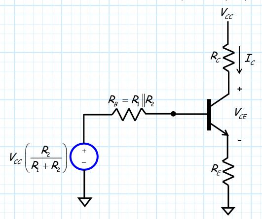
If we **ASSUME** that the BJT is in active mode, then we **ENFORCE** the proper equalities and **ANALYZE** this circuit to find collector current  $I_{\mathcal{C}}$ :
