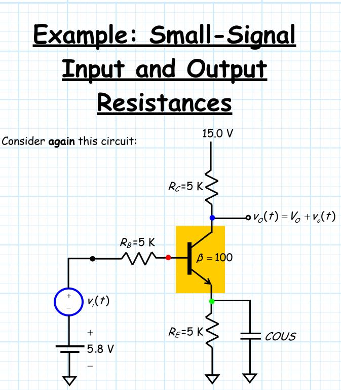
Recall we **earlier** determined the open-circuit **voltage gain**  $A_{o}$  of this amplifier. But, recall also that voltage gain alone is **not** sufficient to **characterize** an amplifier—we likewise require the amplifier's input and output **resistances**!
