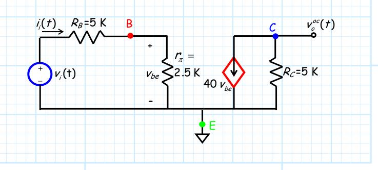
It is evident that the output voltage is simply the voltage across the collector resistor  $R_c$ :
