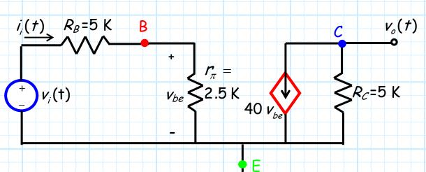
The input resistance of an amplifier is defined as:
