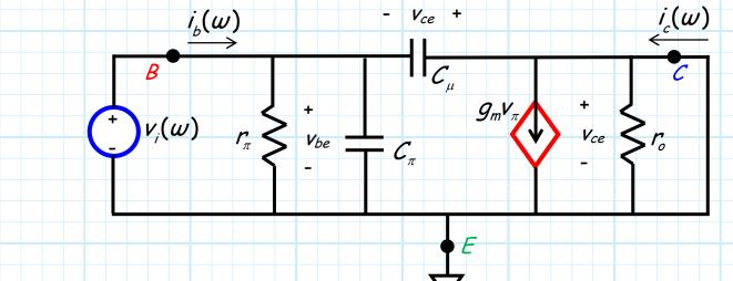
Evaluating this circuit, it is evident that the small-signal base current is:
