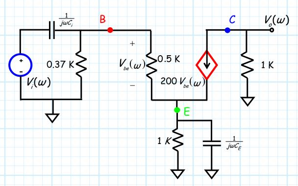
To simplify this analysis, we first determine the **Thevenin's** equivalent circuit of the portion of the circuit connected to the base.
