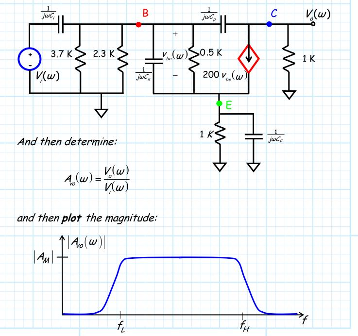
And then from the plot determine the amplifier bandwidth (i.e., determine  $f_L$  and  $f_H$ )?
