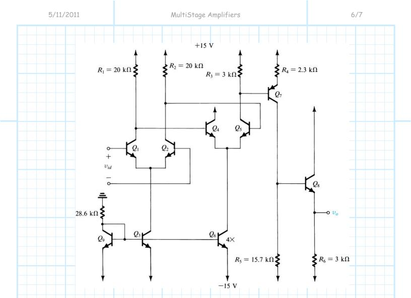
In this multistage circuit,  $Q_9$  forms a current source, and  $Q_3$  and  $Q_6$  complete the current mirror.
