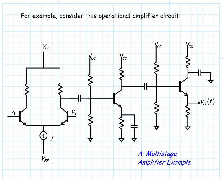
Note the **input** stage is a differential pair, the **gain** stage is common-emitter amp, and the **output** stage is a emitter follower (i.e., common-collector) amp.
