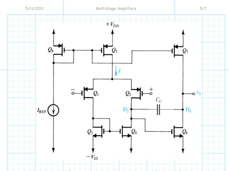
For this example,  $Q_8$  is a current source, with  $Q_5$  and  $Q_7$  parts of a current mirror!
