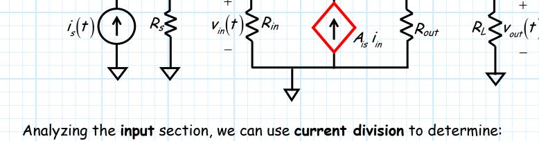
$$\dot{i}_{in} = \left(\frac{R_s}{R_s + R_{in}}\right) \dot{I}_s$$
