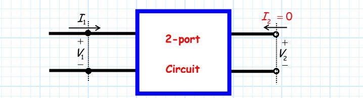
Say we measure/determine the current at port 1 (i.e., determine  $I_1$ ), and we then measure/determine the voltage at the port 2 plane (i.e., determine  $V_2$ ).
