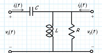
Since this circuit is **linear**, the relationship between **all** voltages and currents can likewise be expressed as **linear operators**, **e**.**g**.:
