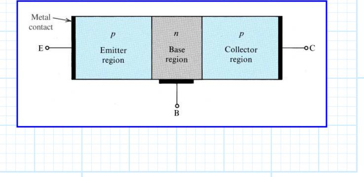
\* For the *pnp* BJT, the **anode** of the **CBJ** is the **collector**, and the **cathode** of the **CBJ** is the **base**.
