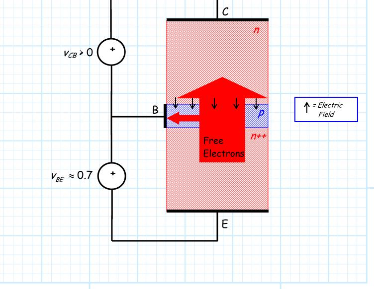
In other words, the large number free electrons in the emitter **diffuse** across the base-emitter junction into the base, then **drift** across the collector-base junction into the collector.
