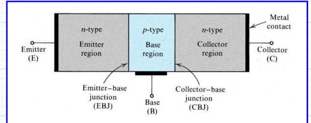
Each of the **three Silicon regions** has one terminal electrode connected to it, and thus the *npn* BJT is a **three terminal** device.
