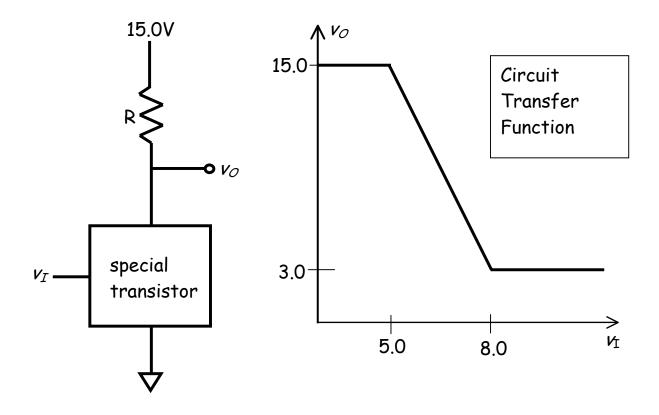
Say we wish to use this circuit as a **small-signal amplifier**. Determine from the transfer function:
