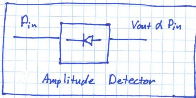
i.e., an Amplitude detector provides an output voltage that is proportional to the input signal power.
