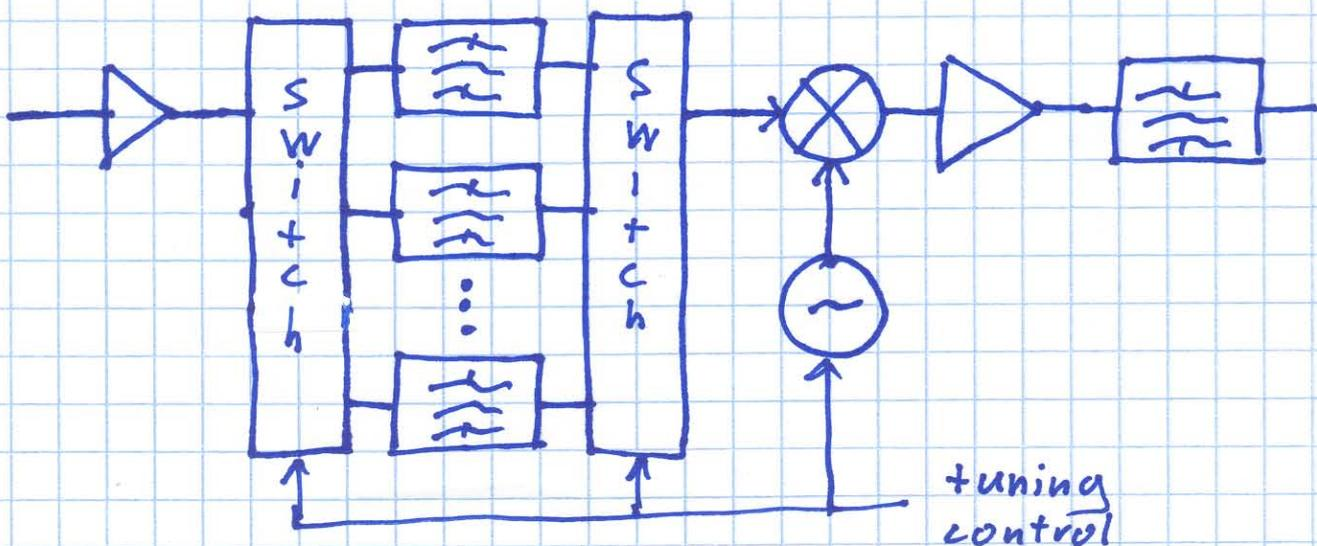
In other words, we use multiple preselector filters to span the Rx bandwidth.
