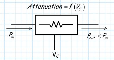
Typical voltage control attenuators can provide attenuation from a minimum of a few dB to a maximum of as much as 50 dB.
