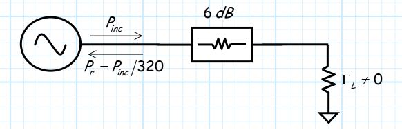
The reason that the return loss improves by 12 dB (as opposed to 6 dB) is that reflected power is attenuated **twice**—once as it travels toward the load, and again after it is reflected from it.
