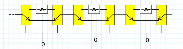
Or we can select **some** attenuators and bypass **others**, thus setting the attenuation to be somewhere in between max and min!
