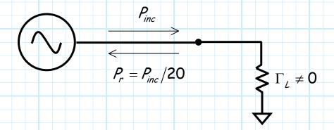
Say we now add a 6 dB pad between the source and the load—we find that the return loss has improved to 25 dB!
