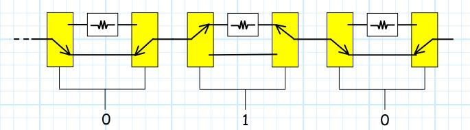
For most digital attenuators, the attenuation of each section has a **different** value, and almost always are selected such that the values in dB are **binary**.
