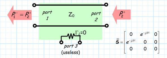
But, this is **not** true for a circulator! If power is incident on port 2, then **no power** will exit port 1!
