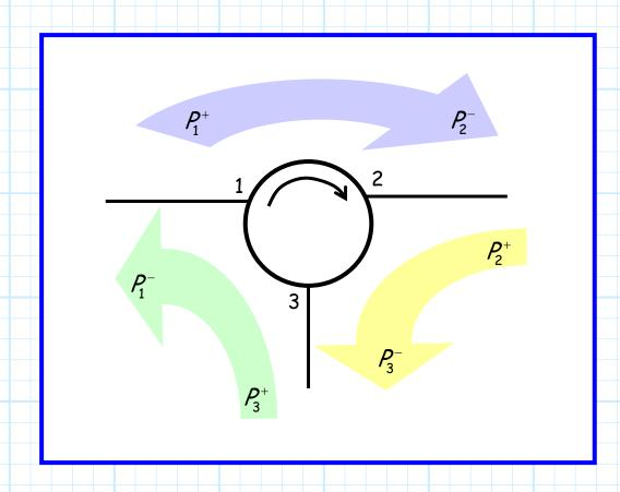
We can see that, for example, a **source** at port 2 "thinks" it is attached to a **load** at port 3, while a **load** at port 2 "thinks" it is attached to a **source** at port 1!
