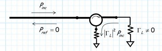
There is **no power** reflected back to the source! Instead, power reflected by the load is **absorbed** by the isolator.
