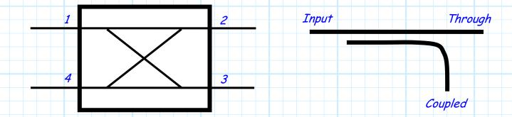
Here are some typical parameters used to specify **technical** the performance of **directional couplers**!
