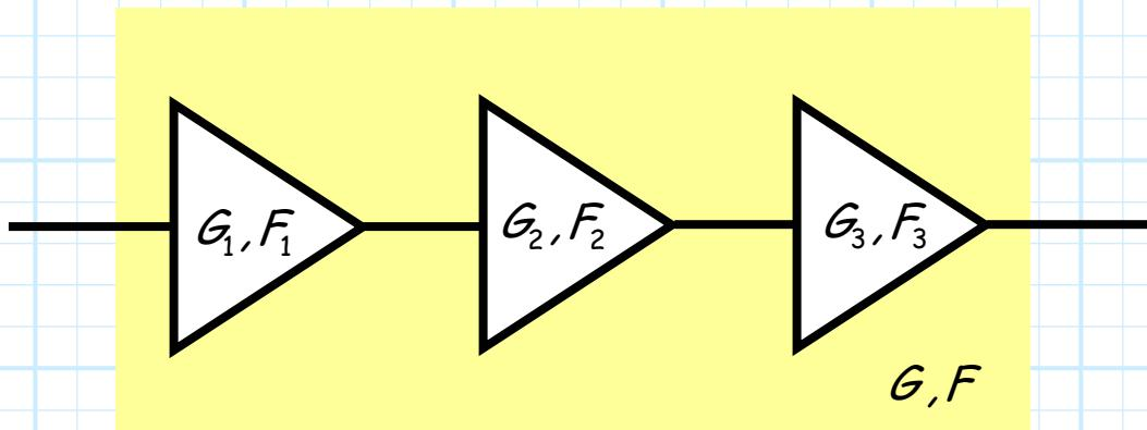
These three devices together can be thought of as **one** new microwave device.
