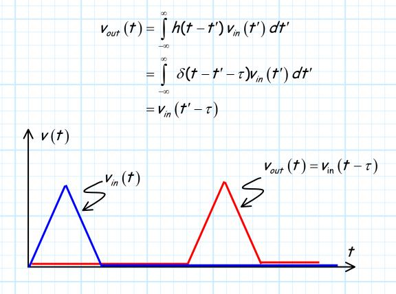
Taking the Fourier transform of this impulse response, we find the frequency response of this two-port network is:
