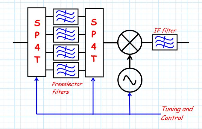
In other words, we use multiple preselector filters to span the desired receiver RF bandwidth. This is particularly useful for wideband receiver design.
