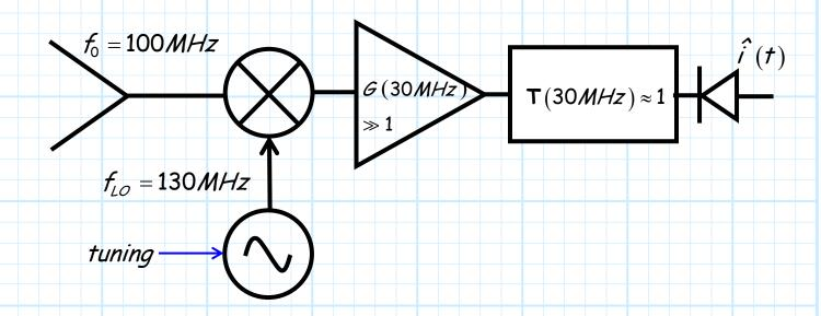
Thus, the desired RF signal will be down-converted to the IF frequency of 30 MHz.
