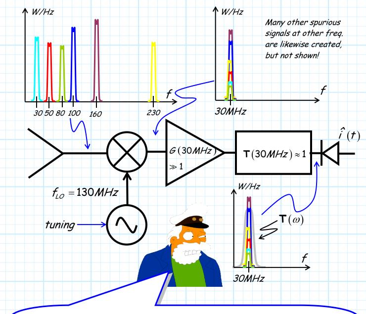
Q: I now see the problem! There is no way to separate the spurious signals at the IF frequency of 30 MHz from the desired station at 30 MHz. Clearly, your hero E.H. Armstrong was wrong about this Super-Heterodyne receiver design!
