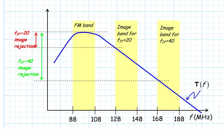
The amount by which the preselector attenuates the image signals is known as the image rejection of the receiver.
