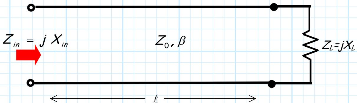
Note that the **opposite** is **not** true: even if the load is **purely resistive** ( $Z_L = R$ ), the input impedance will be **complex** (both resistive and reactive components).
