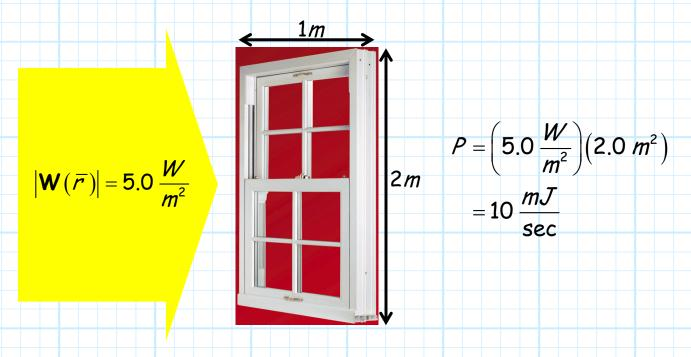
\* The direction of the Poynting Vector indicates the direction of this power flow—the direction of the propagating wave.
