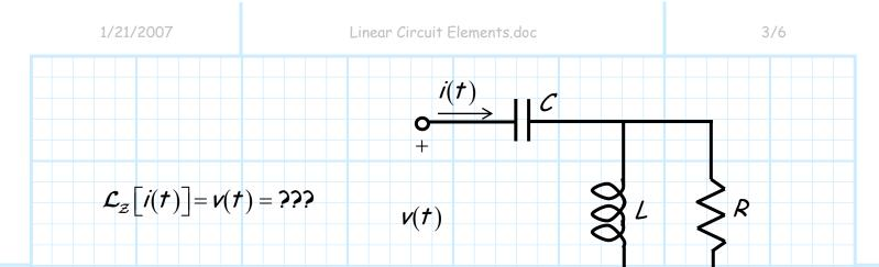
A: It turns out that **any** circuit constructed **entirely** with linear circuit elements is **likewise** a linear system (i.e., a linear circuit).
