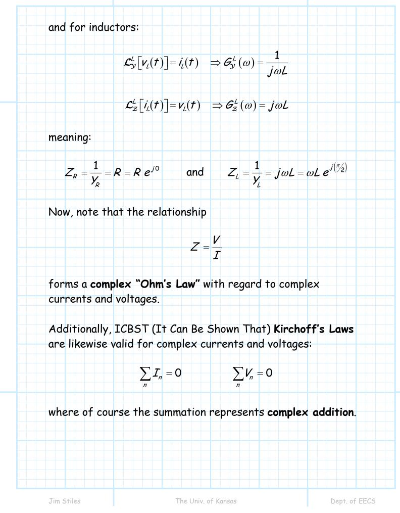
As a result, the impedance (i.e., the eigen spectrum) of **any** one-port device can be determined by simply applying a **basic** knowledge of **linear circuit analysis**!
