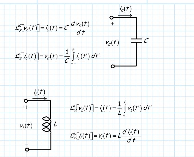
Since the circuit behavior of these devices can be expressed with **linear** operators, these devices are referred to as **linear circuit elements**.
