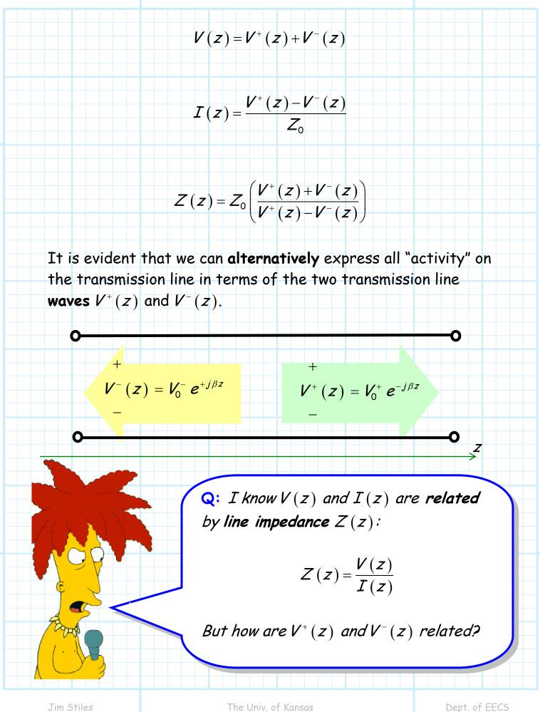
A: Similar to line impedance, we can define a new parameter the **reflection coefficient**  $\Gamma(z)$ —as the **ratio** of the two quantities:
