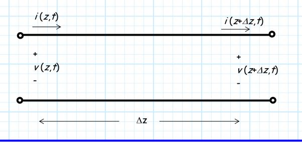
**Q**: Huh ?! Current i and voltage v are a function of **position** z ?? Shouldn't  $i(z,t) = i(z + \Delta z,t)$  and  $v(z,t) = v(z + \Delta z,t)$ ?
