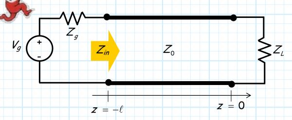
Recall that if  $Z_L = Z_0$ , the **reflected** wave will be **zero**, and the absorbed power will be:
