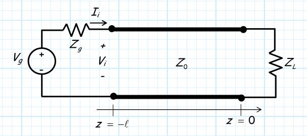
Recall from the telegrapher's equations that the current and voltage along the transmission line are:
