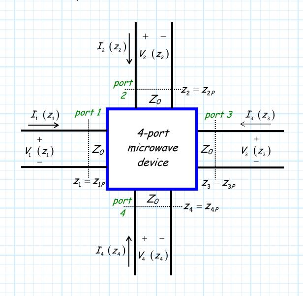
Note in this example, there are four identical transmission lines connected to the same "box". Inside this box there may be a very simple linear device/circuit, or it might contain a very large and complex linear microwave system.
