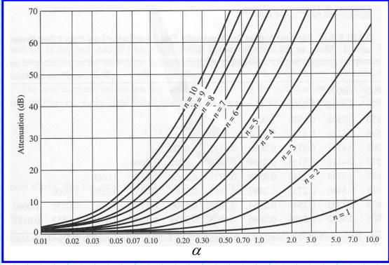
And the normalized attenuation chart for a Chebychev with 3.0 dB of passband ripple is:
