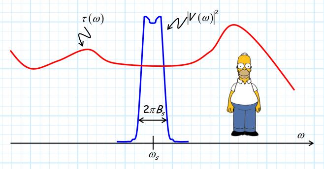
As with the previous case, the phase delay of the filter is **not** a constant. Yet, if this signal were to pass through this filter, it would **not** be distorted!
