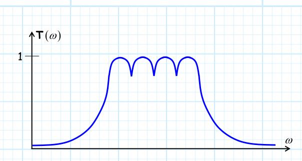
We likewise find that the roll-off can be made steeper by accepting more ripple.
