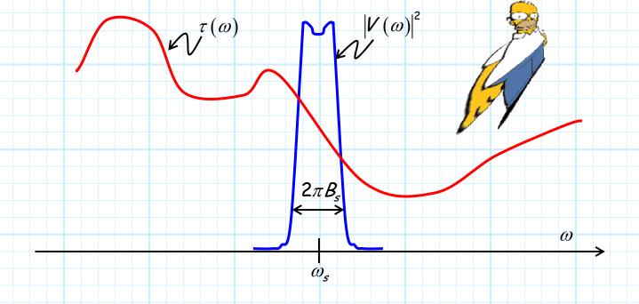
Note that for this case the filter phase delay is **nowhere** near a constant with respect to frequency.
