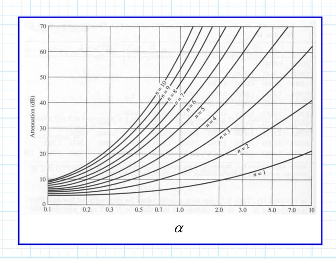
While the normalized attenuation chart for a Chebychev with 0.5 dB of passband ripple is:
