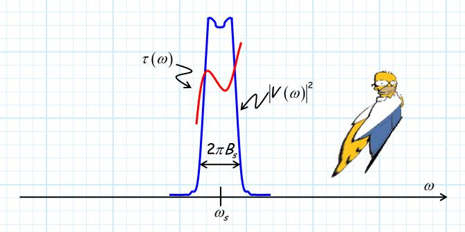
Thus, a narrowband filter (e.g., IF filter) must exhibit a near constant phase delay  $\tau(\omega)$  in order to avoid distortion due to signal dispersion!
