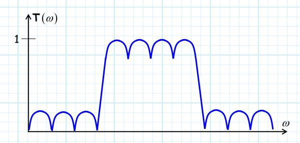
We find that we can make the roll-off steeper by accepting more ripple.
